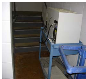
Combustible storage in halls and stairwells can create life hazards
