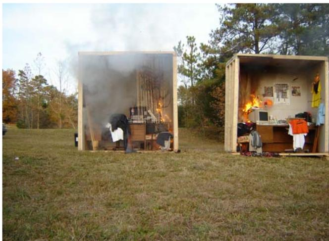
The sprinkler system in the left dorm extinguishes the fire within seconds. Notice the smoke? On the right, the fire continues to burn. Below, Chapel Hill Fire Dept. prepares to extinguish the dorm fire on the right.
