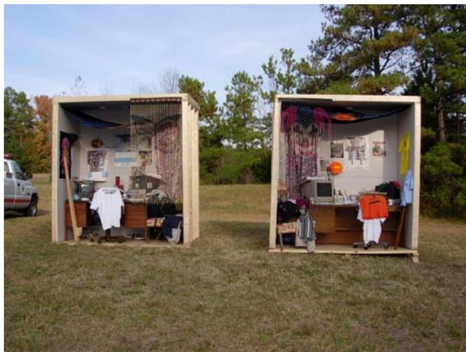
Above, the demonstration dorm on left is sprinkled. On right, non-sprinkled. Below, both fires are started simultaneously.
