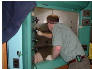
J.D. Moore checks for radioactive contamination prior to release for general use.
