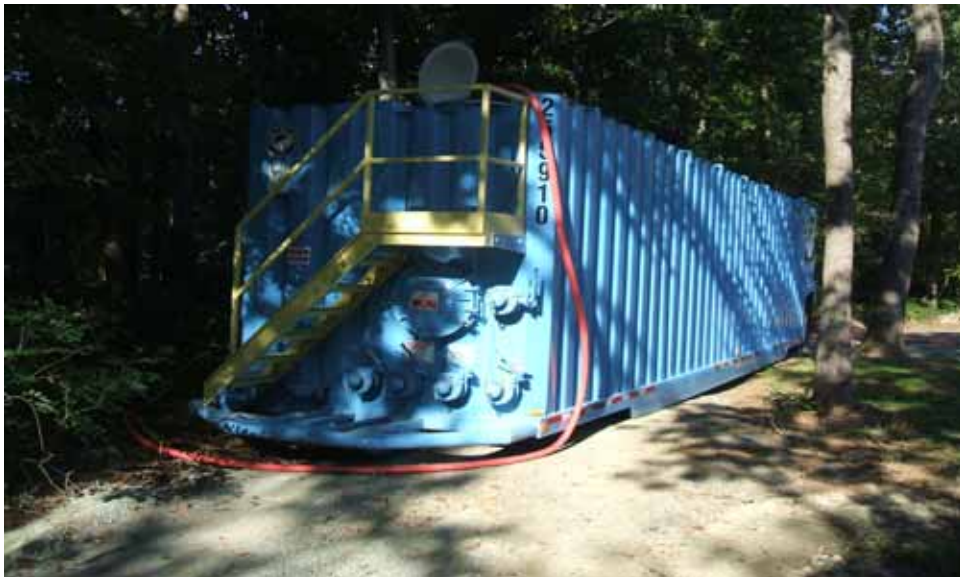
View of tank for temporary storage of treated water
