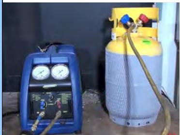
Set the recovery tank on a scale to measure how much refrigerant is removed from the unit, and avoid overfilling the recovery tank. **By law a tank can only be filled to 80 percent capacity**
