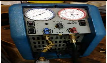
The center yellow hose goes to the suction line of the recover machine marked IN, a dryer should be placed here to help keep contaminants out.
